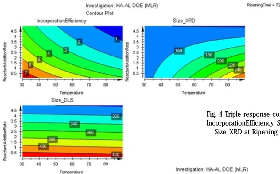
Fig. 4 Triple response contour plot of IncorporationEfficiency, Size\_DLS and Size\_XRD at Ripening time=72h
